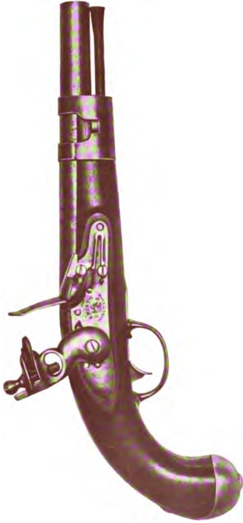
Horse pistol; model of 1813. Length 15½ inches. Length of barrel 9 inches. Caliber, 69. Iron mountings.
